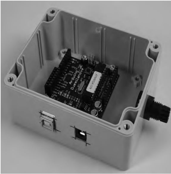
Figure 12-15. Arduino and cable gland mounted in box
