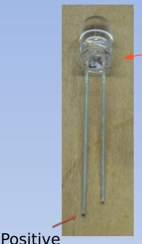
Components can be polarized or non-negative polarized
