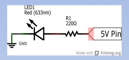
LED should light up when powered by Arduino
