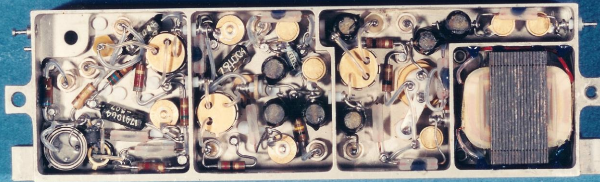
8358760-501 AM Transmitter "B"
