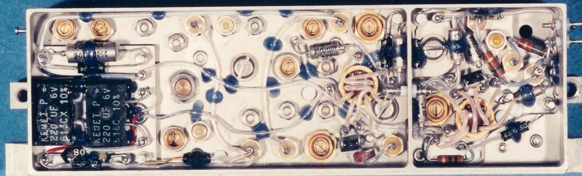
8358760-501 AM Transmitter "B"
