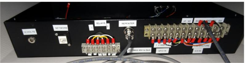
In addition to repeater control, Allstar and Echolink Interface it has two single pole Double throw relays, two temperature sensor inputs, two voltage sensor inputs, and Four GPIO inputs.
